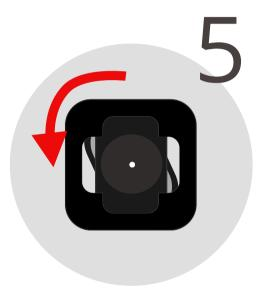
Hold the sensor and then rotate the sensor tool anti-clockwise until you lock the lid
