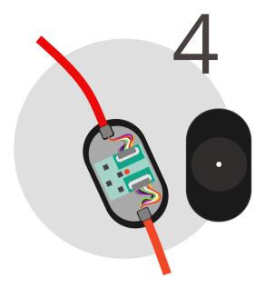
Fold the cables in the plastic case, and make sure the plastic lid does not smash any of the cables
